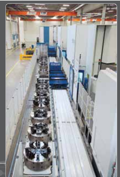
Extremely precise part positioning guaranteed in the FMS, with PIETRO CARNAGHI sub-base coupling for pallet
