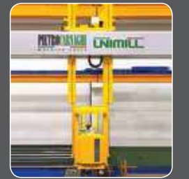
Separate Bridge with fully movable operator platform in machining area
