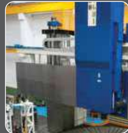
Continuous W axis with mechanical locking system for high rigid turning
