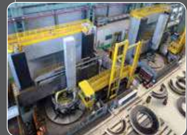
Fully controlled operator platform moving on 3 axis
