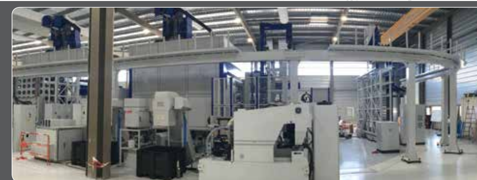
Tool Management System: shuttle to handle thousands of tools connecting machine tool magazines
