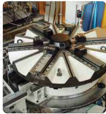
Special design table for chip evacuation
