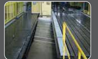
Automatic telescopic walkable bridge for operator operations
