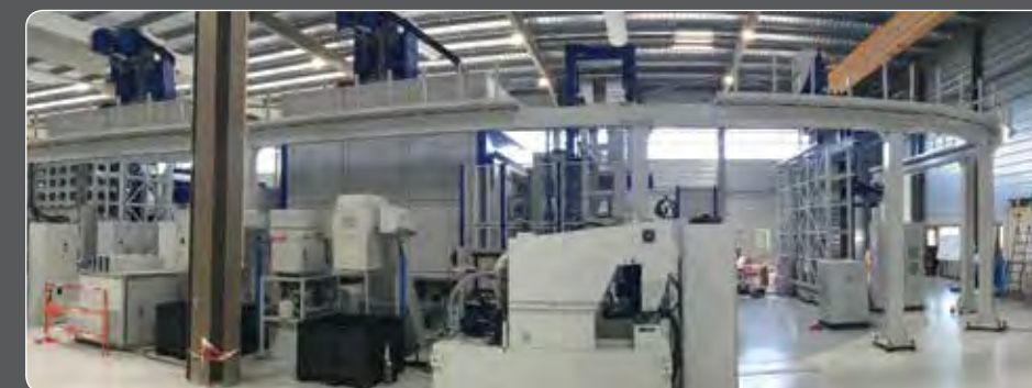
Tool Management System: shuttle to handle thousands of tools connecting machine tool magazines
