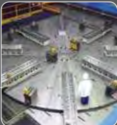
Fully Automatic accessory change and travelling robot for tools
