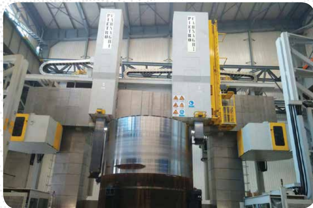
Continuous W axis with mechanical locking system for high rigid turning
