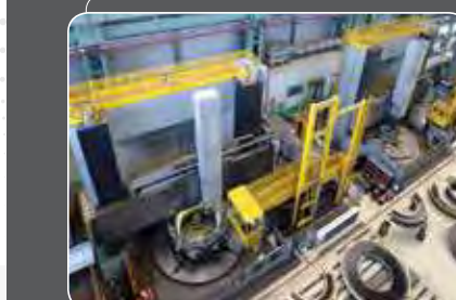
Fully controlled operator platform moving on 3 axis
