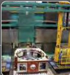
Separate Bridge with fully movable operator platform in machining area
