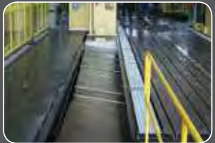
Automatic telescopic walkable bridge for operator operations
