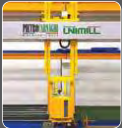
Separate Bridge with fully movable operator platform in machining area
