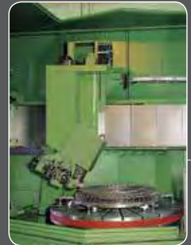
Independent grinding carriage (to be added to turning carriage)
