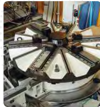
Special design table for chip evacuation
