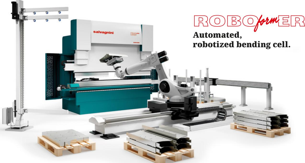
Depending on the configuration chosen, consists of a B3 press brake, a robot and a number of devices for automatic sheet metal handling.
