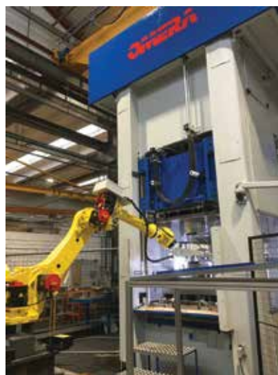
Pressa idraulica OPI.M 250 asservita da Robot / Hydraulic press OPI.M 250 with Robot
