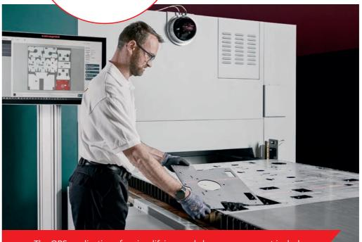
The OPS applications for simplifying workshop management include PDD, which supports the operator via the monitor for manual part separation and sorting, and LPG, which laser-guides the operator in the pick-up sequence.
